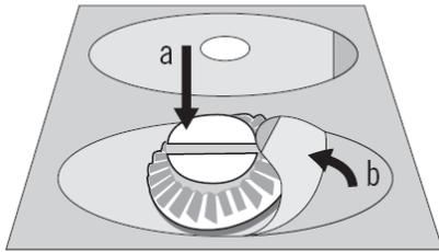
The blocking piece is stuck onto the film and is pulled off with it. The anti-slip film and the blocking piece are then applied to the convex side of the lens together.
